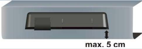
Mount the sensor at a maximum height of 5 cm from the bottom line of the door controller.
