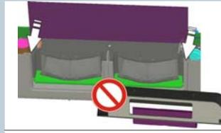
Make sure to introduce the prism into the guiding grooves in front of the lenses and not into the cover!
