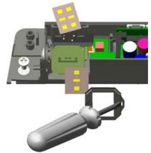
Touching the antenna patches will not cause any damage!
